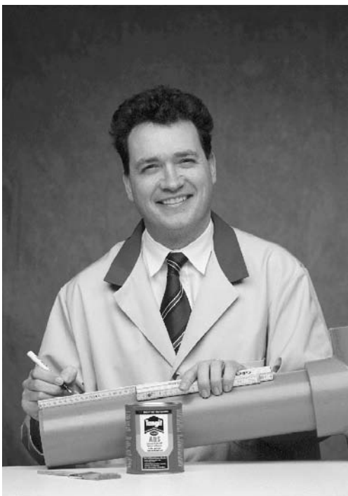
Marking the jointing length
