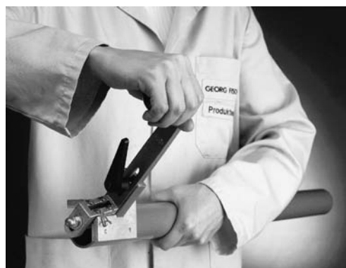
Chamfering the pipe
