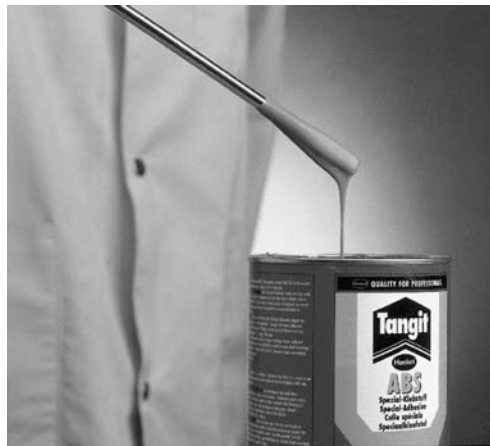
Checking the cement
