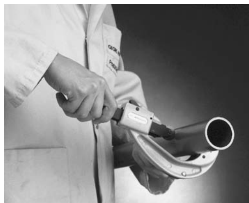
Cutting the pipe to length
