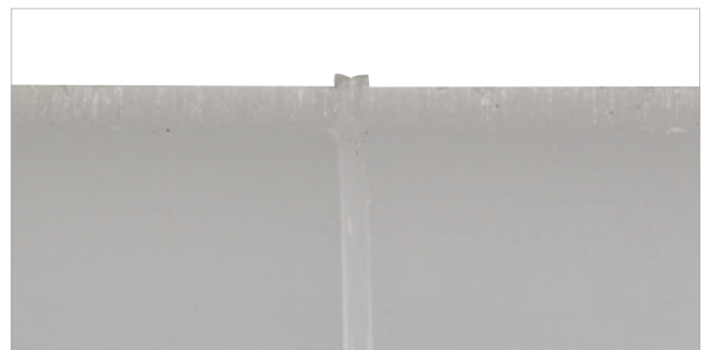
Lateral cut of IR (infrared) welding
