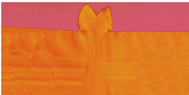
Macro-image of IR (infrared) welding
