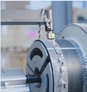
Peel the ends of the pipe and fitting type B and clean the fusion zones of the fitting and pipe using a clean cloth.
