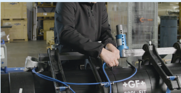
Connect the welding cables to the welding contacts of the fitting and weld according to the instruction manual.
