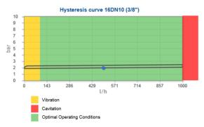
In case the flow rate is exceeding the maximum value (see graphic below) of the diagram the valve dimension is too small and the next larger valve should be taken into consideration, since the valve would most likely lead to cavitation.
