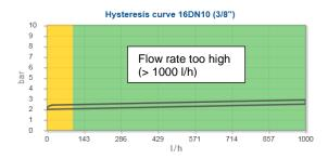
In case the flow rate is too low (see graphic below) the valve is too large and therefore a smaller valve should be chosen for the application. Valves too small lead to vibrations and consequently reduce valve lifetime.
