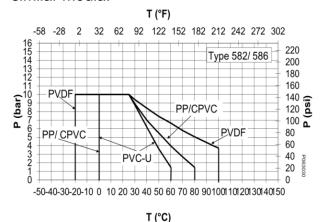
**P** permitted pressure in bar, psi **T** temperature in °C, °F
